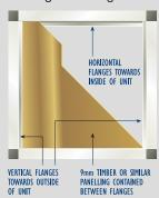
I. In this assembly, the flanges on the top and bottom (horizontal) tubes are nearest the inside of the unit. The vertical tube flanges are nearest the outside of the unit. The vertical panel is locked against movement in any
