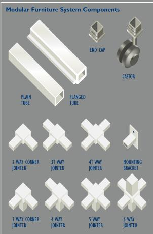
These components are available for 20mm and 25mm profiles. Standard tube finishes are plain milled, anodised silver or powder-coated in white or bronze. Tubes may also be painted with approved enamel finishes. Jointers are made from heavy-duty injection-moulded plastic in black or white.
