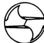
A drill with web properly thinned
