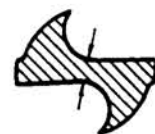
Web thickness near point
